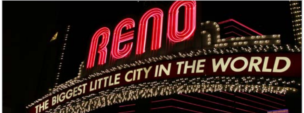
As part of the comprehensive lighting upgrade project, Ameresco replaced over 2,000 incandescent 11 Watt light bulbs with 2 Watt LED light bulbs.
